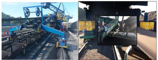
Thanks to radar technology, factors such as coal dust, snow, rain, fog, lack of lighting, etc. do not affect the operation of the system
