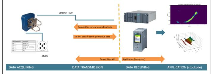
Therefore, the complete system includes 3D Radars from Kymati, a PLC controller (in an industrial housing) and GSK Industry software for data cloud analysis.
